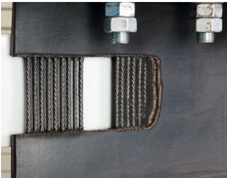
High-capacity steel wire belt with wire-free zones for fixing the buckets
