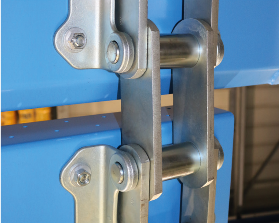
BEUMER central chain bucket elevator
